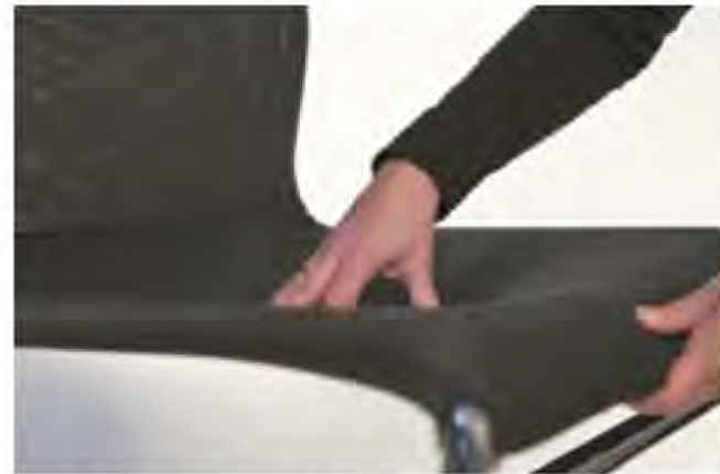
The frame is upholstered with the fabric sack, then fixed
