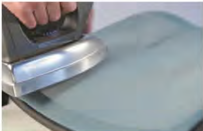
The fabric shrinks with heat to the defined shape and tension
