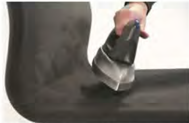
The upholstery cover shrinks with heat in its shape and tension
